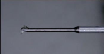
Boron cantilever & Aluminum body
