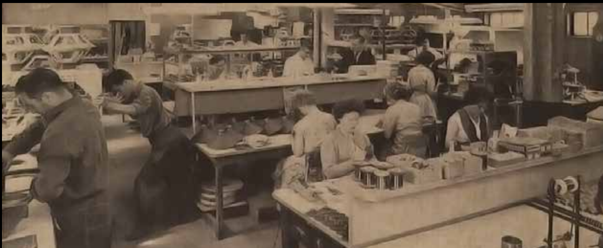
General view of the voice coil winding and speaker assembly department.
