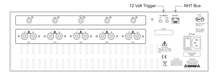
The Power<sup>5</sup> has both 12 volt trigger connections and the NHT Bus connection. A 12 volt trigger cable is supplied with the Power<sup>5</sup>.
