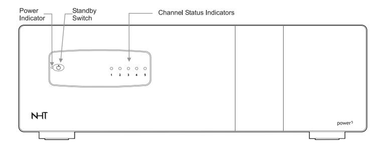
Power indicator - This LED is GREEN when the Power<sup>5</sup> is on and AMBER when it is in standby mode.
