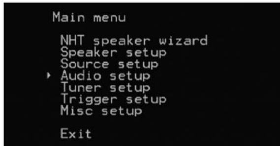
The Audio setup menu lets you select Favorite mode setup, Dolby/DTS setup, Preset setup as well as "general" tone controls for treble, bass, LFE level, and Reverb.
