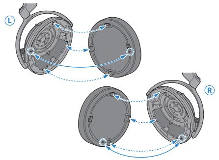
**3** Hold the earpad and rotate clockwise while attaching the earpad onto the headphones.
