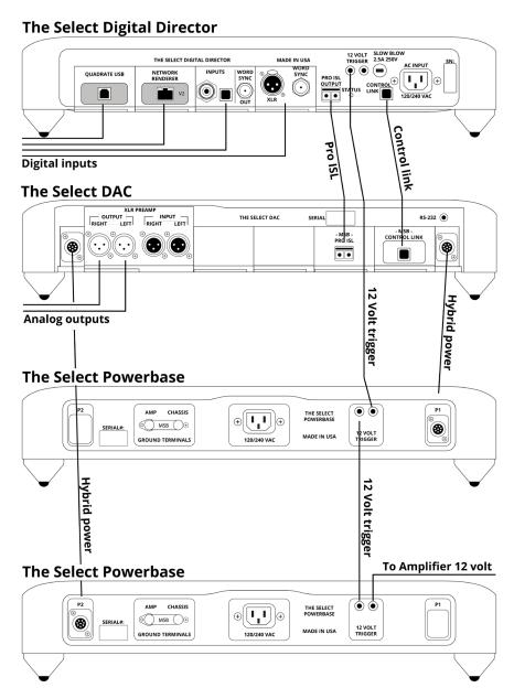
When installed properly, your system should look like the example above. The digital inputs installed in your digital director may vary depending on what sources are in your system, However; the only modules that should be installed in the DAC will be the provided Pro ISL and Control Link modules as well as any analog input modules you may have in your system.
