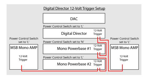
The diagram above is only a visual example and the actual connections may vary in your system. The specific order in which the units are connected does not affect how the 12 volt connections will function. The only requirements are that each unit is connected to a 12 volt trigger port of another unit in the chain. Only one unit is set to the normal 'N' position while all other units are set to the linked 'L' position.
