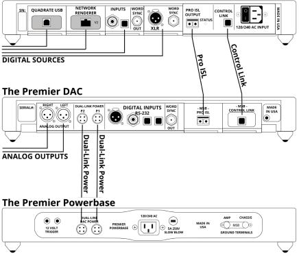
When installed properly, your system should look like the example above. The digital inputs installed in your digital director may vary depending on what sources are in your system, However; the only modules that should be installed in the DAC will be the provided Pro ISL and Control Link modules as well as any analog input modules you may have in your system.
