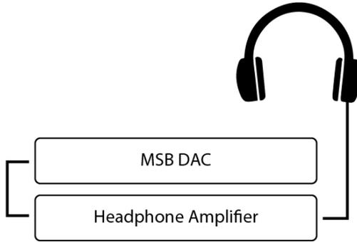
Connect the "Analog Outputs" located on the back of your MSB DAC to the "Analog Inputs" located on the back of your headphone amplifier.
