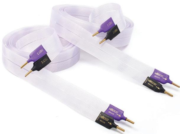
**A**lso insulated with FEP, this precision micro-mono-filament constructed cable includes twenty-two conductors and is made from sixty micron, silver-plated 99.99999%, solid core OFC.
