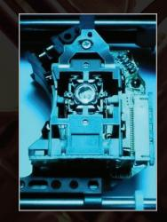
dramatically improve tracking. This enclosure is mounted on the aforementioned dual-rail apparatus which prevents any off-axis tilling when the lens moves. All of these features combine to ensure quieter disc rotation.
