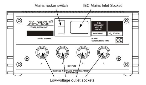
Using any of the four accessory 3-pin DIN leads supplied, plug one end into the low-voltage inlet socket on your X <sup>V3</sup> Series unit, and the other end into one of the X-PSU <sup>V3</sup>'s outlet sockets on the rear panel.
