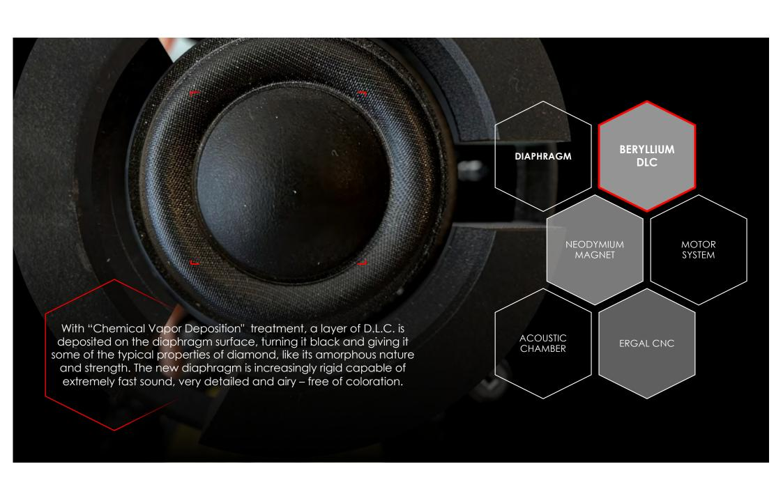
With "Chemical Vapor Deposition" treatment, a layer of D.L.C. is deposited on the diaphragm surface, turning it black and giving it some of the typical properties of diamond, like its amorphous nature and strength: the new diaphragm is increasingly rigid so its resonance frequency is moved way higher: the beryllium extremely fast, detailed and airy sound is kept – but now it is free of any coloration.
