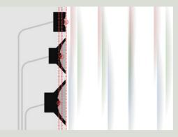
In a normal speaker the acoustic centres of the treble, midrange and bass are not aligned.
