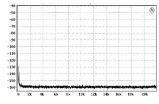
The results are limited by the capabilities of the measuring equipment and noise floor lays at  $-160 \, \text{dB}$  or even lower. There are visible peaks at 50Hz and 100Hz which are caused by limits of the measuring instruments. However, they are at a level of  $-130 \, \text{dB}$  and  $-140 \, \text{dB}$ .
