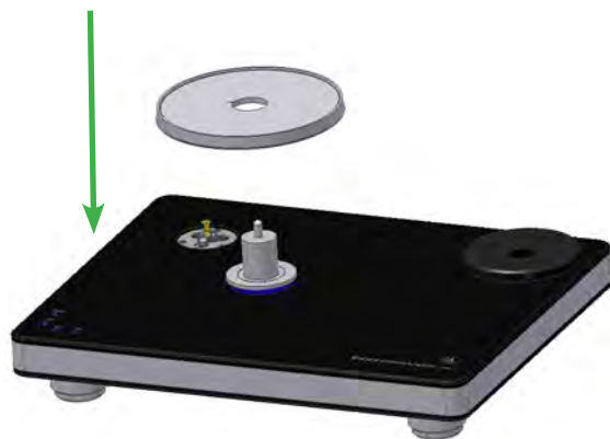
Pic. 7: Setting the sub-platter
