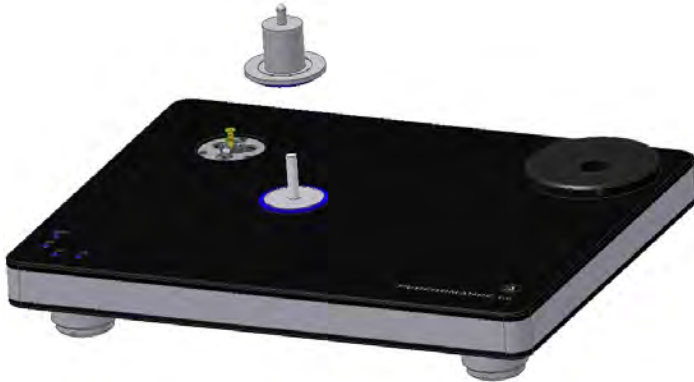
Pic. 6: Fitting the bearing upper part
